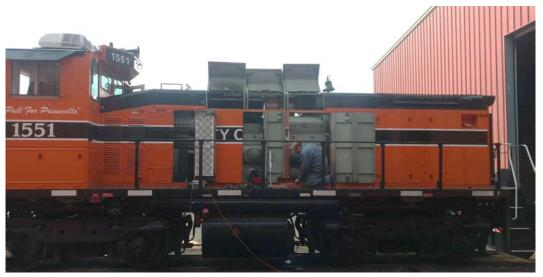
Injector getting replaced in the locomotive at the freight depot.
