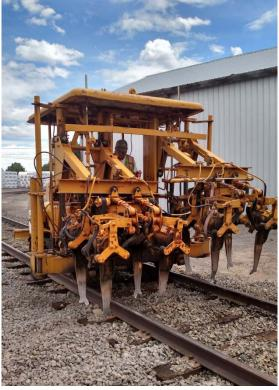
Tamping and leveling a newly constructed yard spur at the Prineville Freight Depot.
