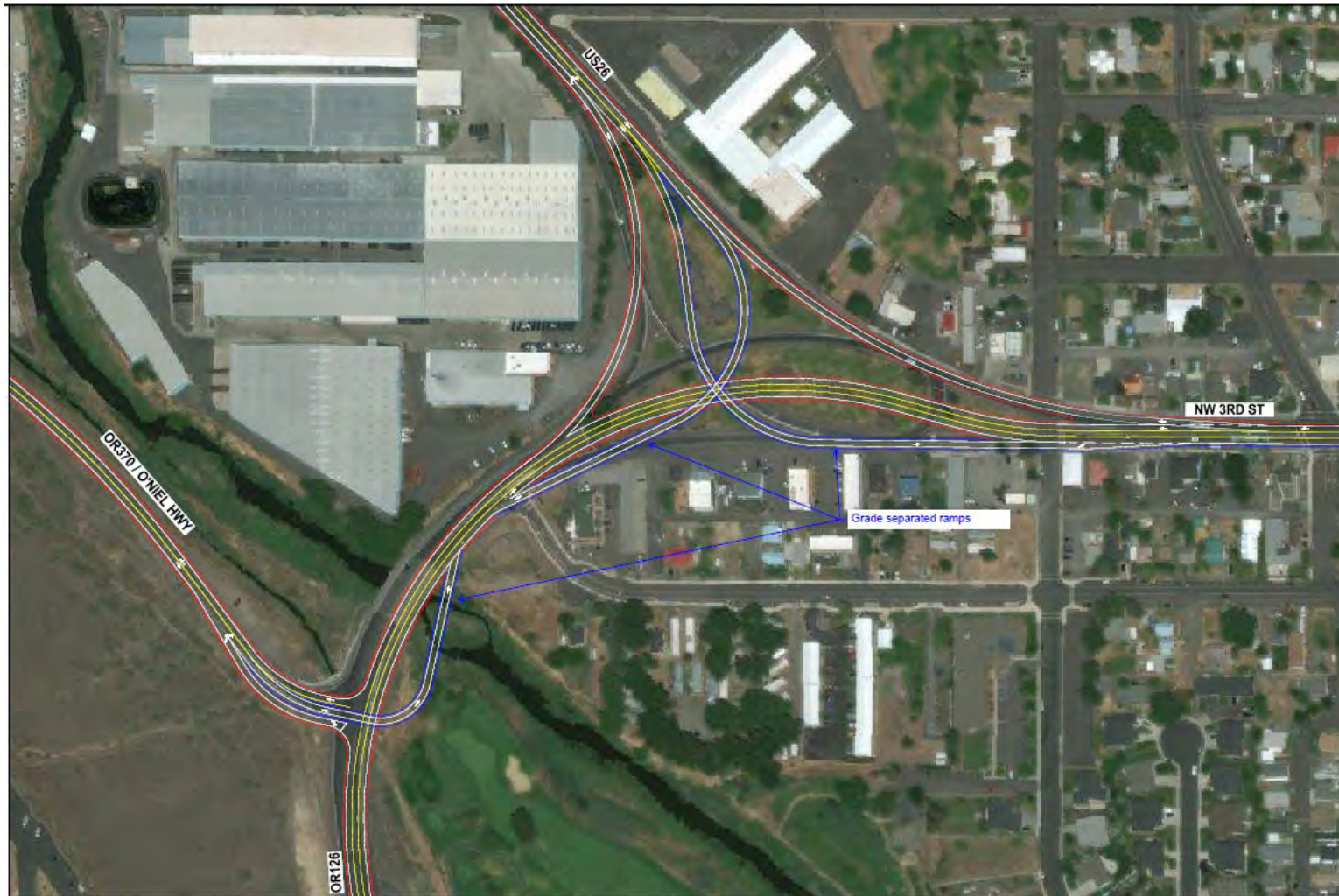
Figure 3. Alternative 4: Grade Separation
